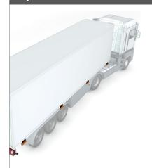
The new revision provides for that all side markers must flash in simultaneously with the direction indicator from the rear lamp, or you must mounted three CAT 5 direction indicators on each side.
